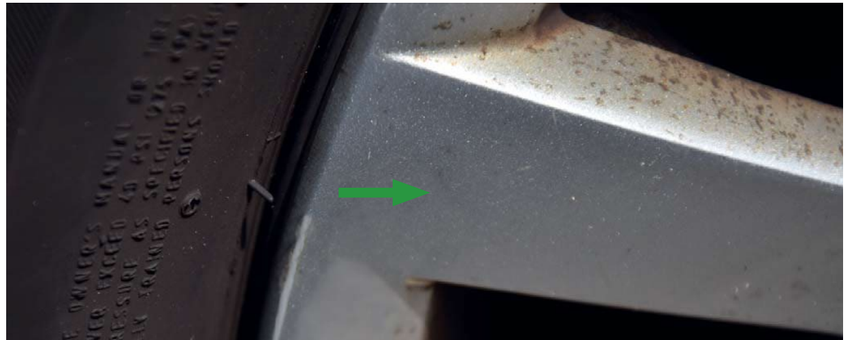
Minor scratch on the wheel trim
