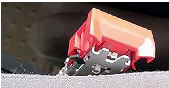
Damaged belt whip
