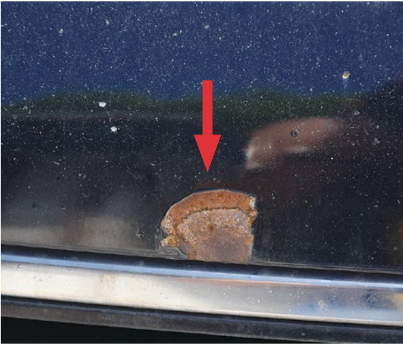
Large stone chip with rust
