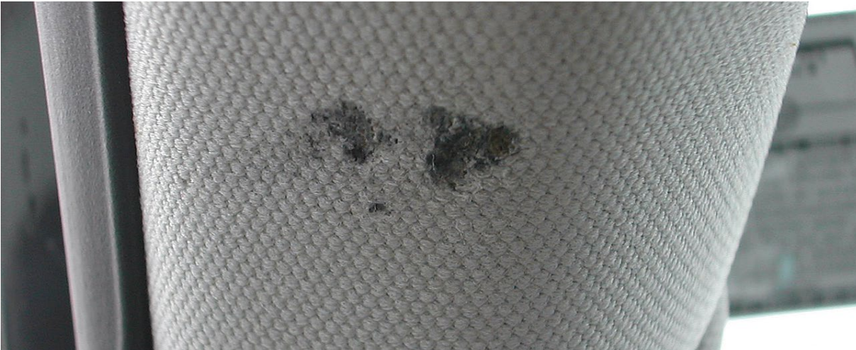
Hole in interior lining
