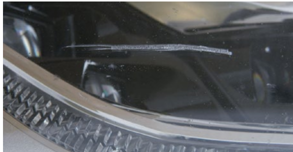
Heavily scratched headlight
