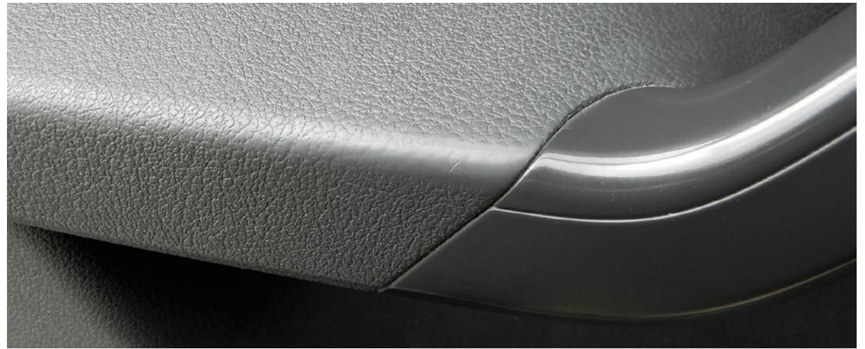
Slightly worn out interior lining
