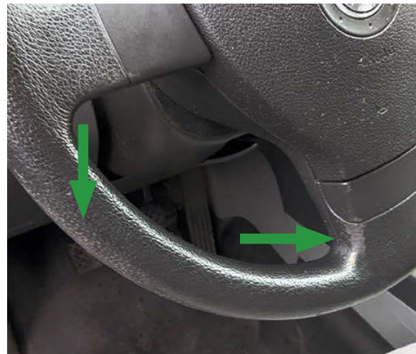
Worn out steering wheel
