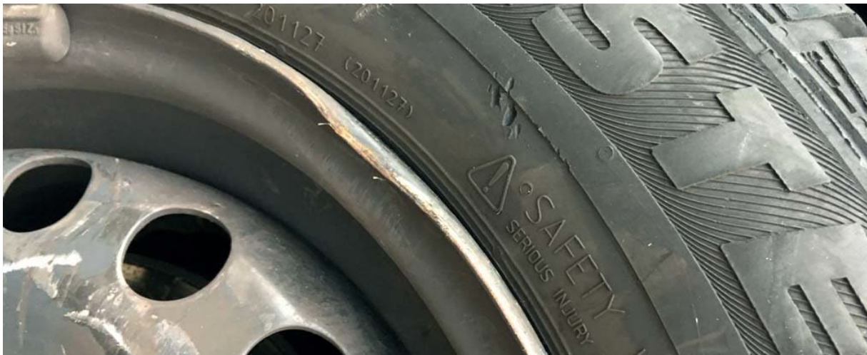
Deformed steel rim
