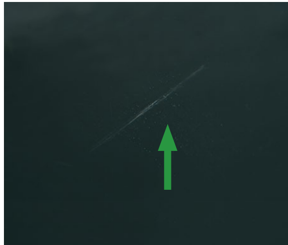
Small scratch, polishable < 1 cm
