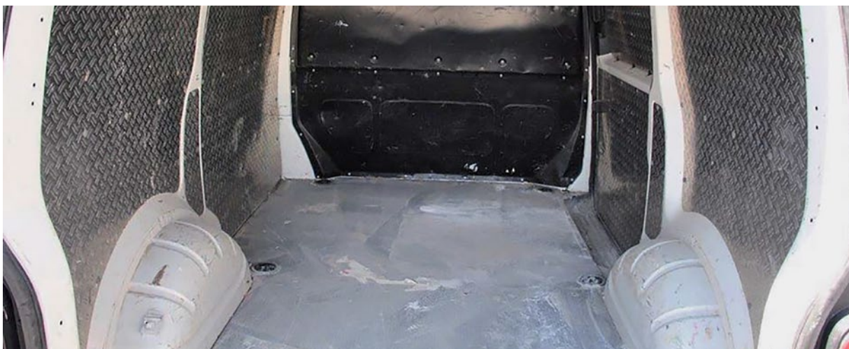
Unacceptable signs of wear on the loading area
