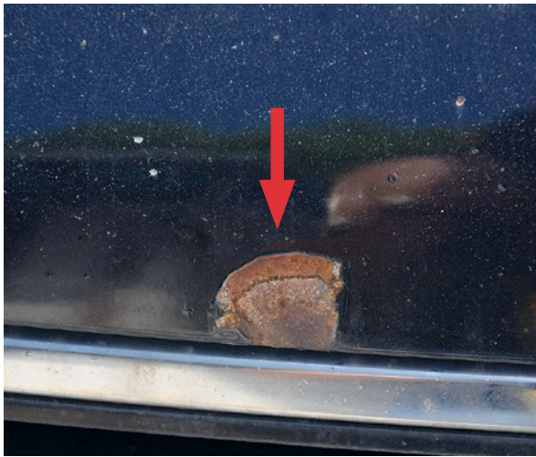
Large stone chip with rust
