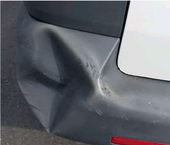
Strongly deformed bumper
