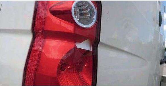
Crack in tail light
