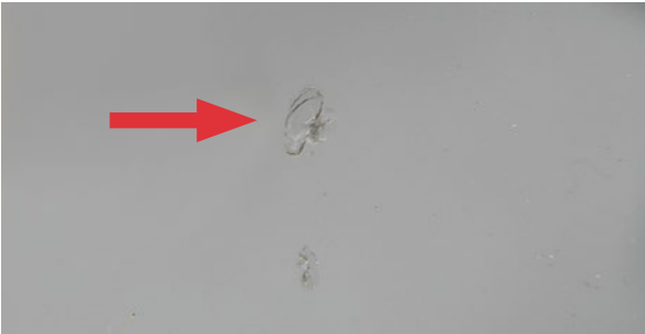
Poorly repaired stone chip on windscreen
