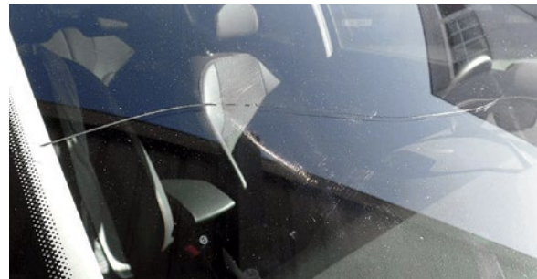
Crack in the windscreen
