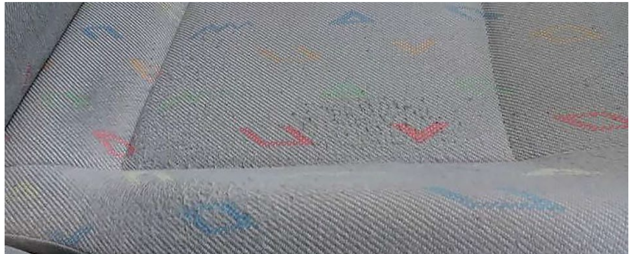
Seat with normal signs of wear
