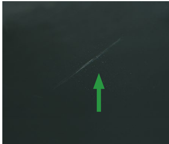
Small scratch, polishable < 1 cm
