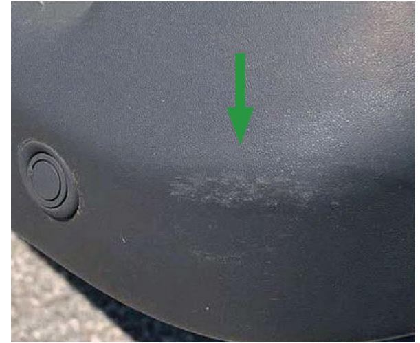
Plastic bumper slightly scratched
