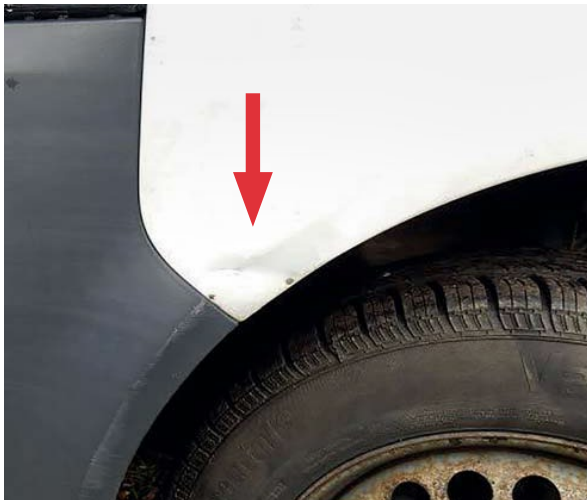
Heavily damaged fender
