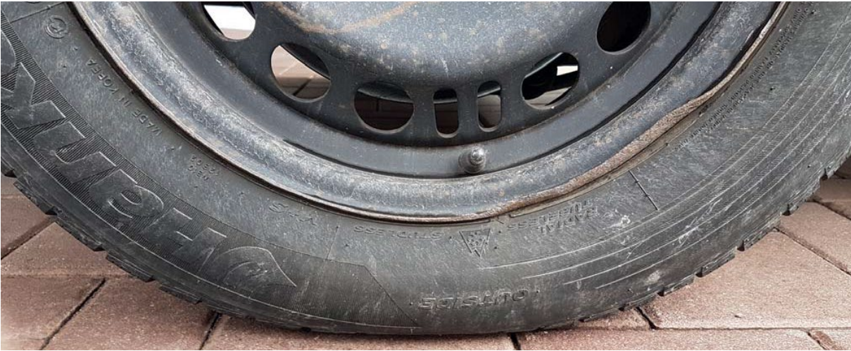
Damaged steel rim
