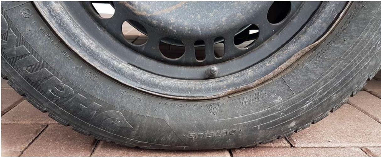
Damaged steel rim
