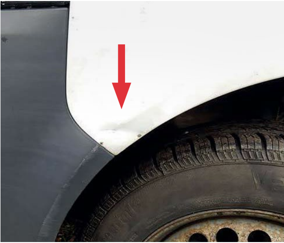
Heavily damaged fender
