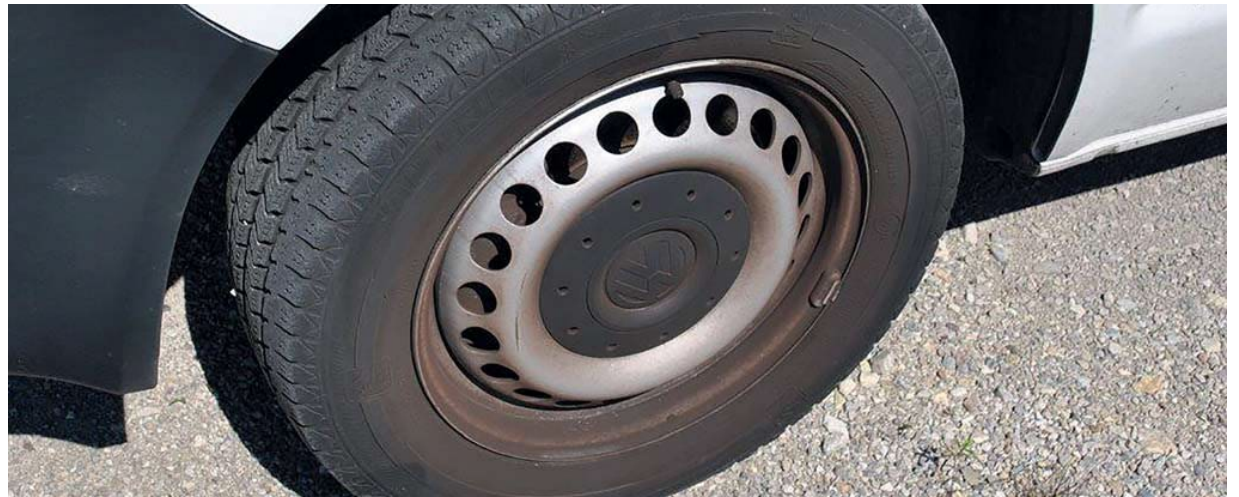
Slightly rusty rim but not damaged
