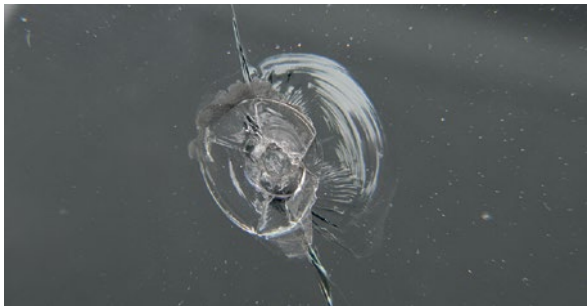
Crack in the windscreen
