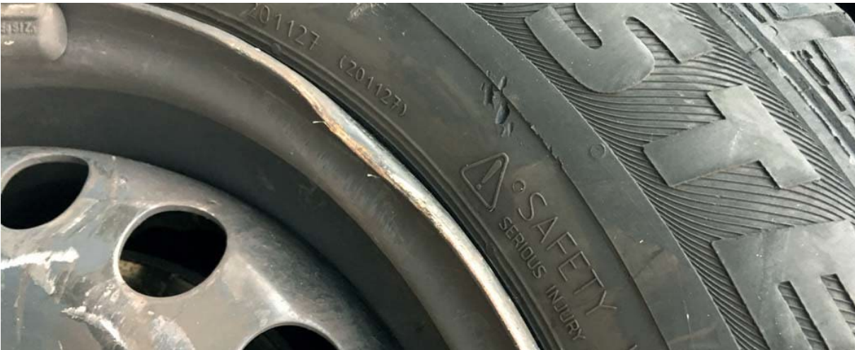
Deformed steel rim
