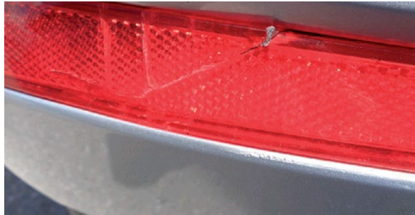
Broken small glass parts
